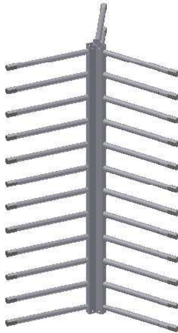
Figure 3-5. Standard Rotor Arms, (Powder Coat, Stainless or Galvanized)
