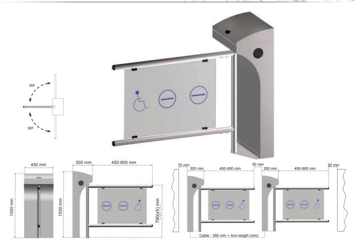
**Power Requirements** : 110/220V. 60/50Hz. AC (%±10) 24V. DC at standby ~11W. max. ~65W.
